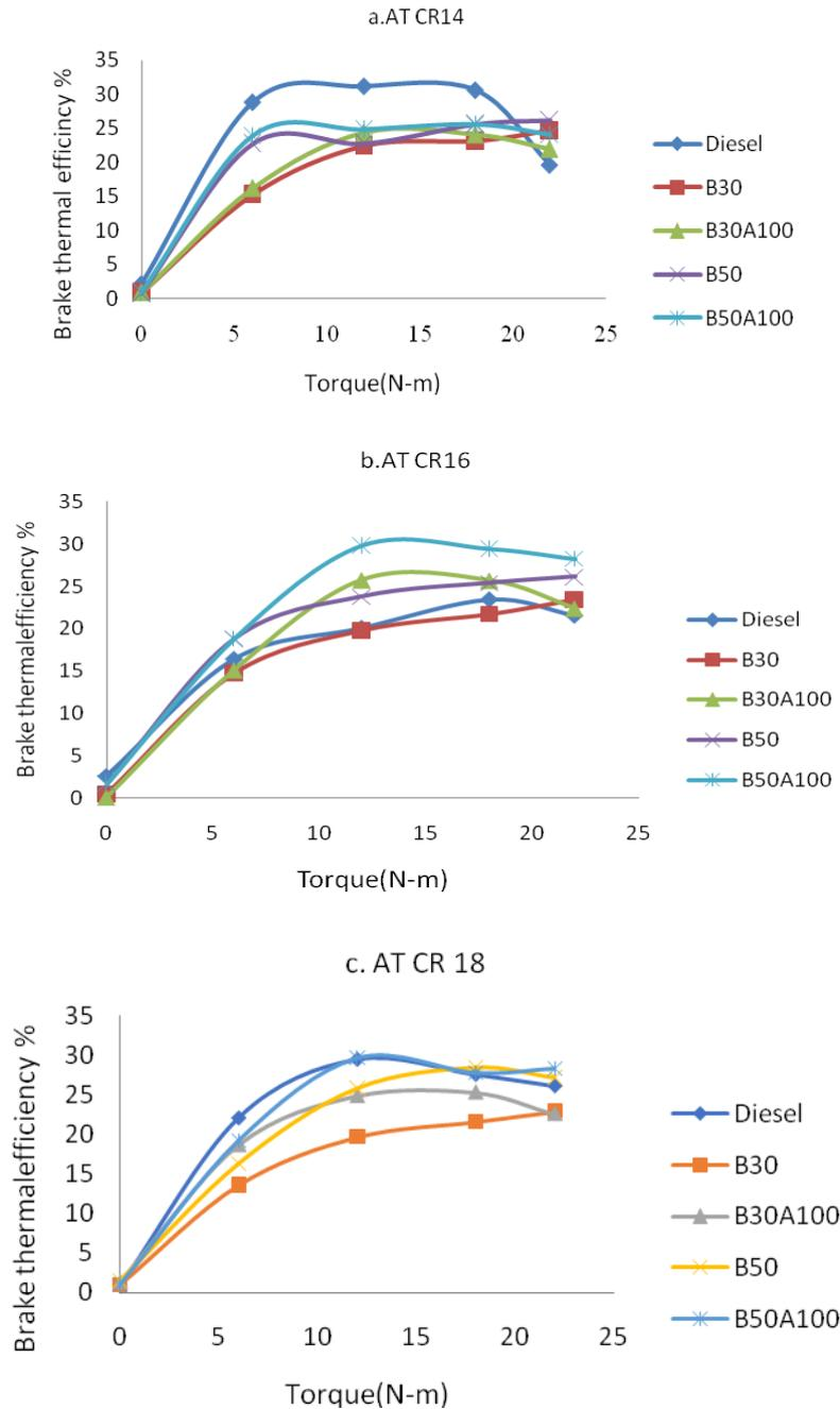
**Figure 1: Variation of break thermal efficiency with Torque at different compression ratios**
