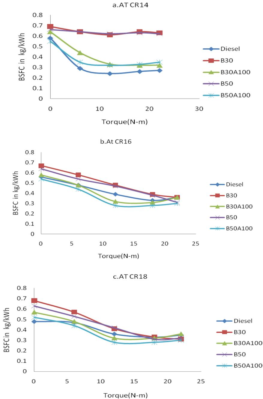
**Figure 2: Variation of Brake specific fuel consumption with torque at different compression ratios**
